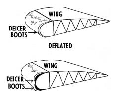
Figure 1: Pneumatic Deicing Boot
