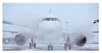
Figure 2: Chemical De-Icing on the Ground
